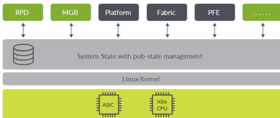
Figure 2: Cloud/Carrier-Class Junos OS Evolved Network Operating System
