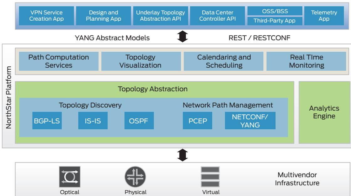
Figure 1. NorthStar architecture
